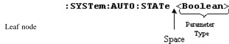
Figure 6 Command Header with Parameter
